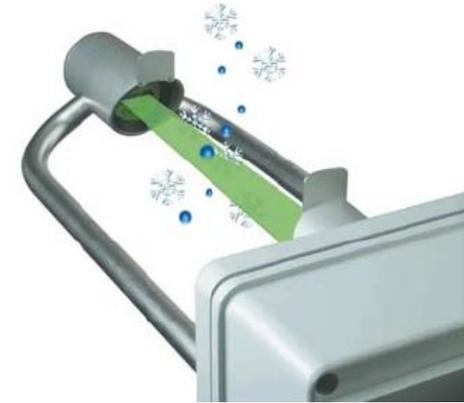
The results of the tests highlights that the instruments in some cases attribute the drops to the upper class of diameter, inducing a overestimation of rainfall intensity.
