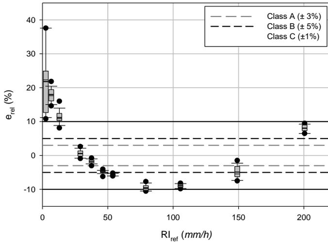
Adopting a calibration curve of the drop volume, the instrument performance increase and fulfil the Class A requirements for almost the full operating range.
